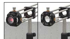
Click to Enlarge [APPLIST] [APPLIST] The CXY1QF integrated into a cage system. A Frosted Glass Alignment Disk in the quick release plate helps line up the beam with the optical axis.
