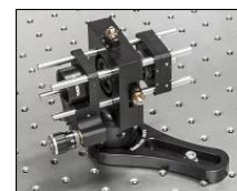
Click to Enlarge Figure 4: Spatial Filter System
