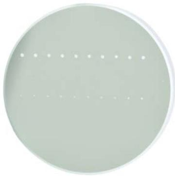
The photograph above is a protected aluminum-coated mirror after LIDT testing. In this particular test, it handled  $0.43$  J/cm<sup>2</sup> (1064 nm, 10 ns pulse, 10 Hz,  $\varnothing$ 1.000 mm) before damage.
