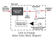
continuously attenuating and modulating the laser output using the liquid crystal retarder and integrated polarizer. Unlike most attenuators available, Noise Eaters attenuate the laser power rapidly without the use of any mechanical components. The noise eater's attenuation capabilities can be controlled via the onboard potentiometer or electrical modulation input.
