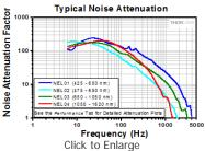
Noise Attenuation Factor is the Ratio of Noise Amplitude Before and After the Noise Eater Thorlabs.com - Noise Eaters / Laser Amplitude Stabilizers
