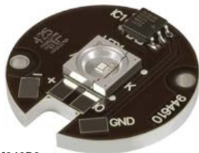
M340D3 340 nm LED, Power Output ≥ 53 mW
