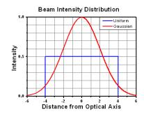
Now compare the maximum power density to that which is specified as the LIDT for the optic. If the optic was tested at a wavelength other than your operating wavelength, the damage threshold must be scaled appropriately. A good rule of thumb is that the damage threshold has a linear relationship with wavelength such that as you move to shorter wavelengths, the damage threshold decreases (i.e., a LIDT of 10 W/cm at 1310 nm scales to 5 W/cm at 655 nm):
