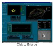
LMM-15X-UVV Interferogram with Measured Seidel Coefficients
