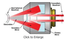
The wavefront is partially obscured by the secondary mirror
