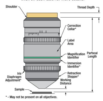
This microscope objective serves only as an example. The features noted above with an asterisk may not be present on all objectives; they may be added, relocated, or removed from objectives based on the part's needs and intended application space.
