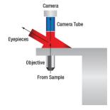
When viewing an image with a camera, the system magnification is the product of the objective and camera tube magnifications. When viewing an image with trinoculars, the system magnification is the product of the objective and eyepiece magnifications.
