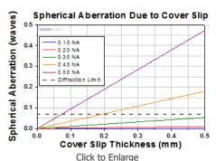
The graph above shows the magnitude of spherical aberration versus the thickness of the coverslip used for 632.8 nm light. For the typical coverslip thickness of 0.17 mm, the spherical aberration caused by the coverslip does not exceed the diffraction-limited aberration for objectives with NA up to 0.40.
