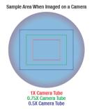
As the magnification increases, the resolution improves, but the field of view also decreases. The dependence of the field of view on magnification is shown in the schematic to the right.
