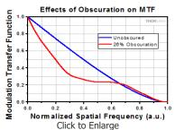
**Figure 4:** Obscurations impact the modulation transfer fuction (MTF) and image contrast. The theoretical MTF shown here is for a central circular obscuration with three straight spider vanes.
