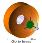
Figure 2: This ray trace diagram illustrates the optics and obstructions in a reflective objective with three straight spider vanes.
