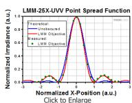
**Figure 3:** This irradiance graph includes point spread functions and measured data of a gaussian beam through a reflective objective with 26% obscuration. The x-axis is the normalized distance from the theoretical maximum to the first minimum of the reflective objective.
