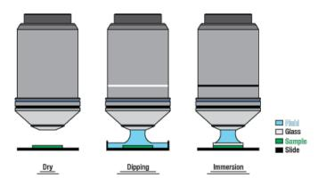
Objectives can be divided by what medium they are designed to image through. Dry objectives are used in air; whereas dipping and immersion objectives are designed to operate with a fluid between the objective and the front element of the sample.
