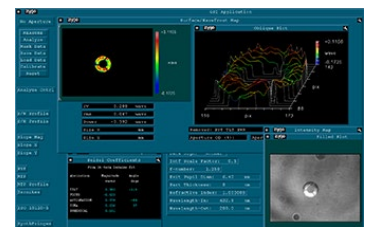
Click to Enlarge LMM40X-UVV Interferogram with Measured Seidel Coefficients
