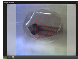
Click to Enlarge A predefined triangle scan pattern can be loaded and scanned in the software. The size can be changed with the Zoom feature.
