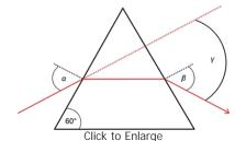
The diagram above shows the relationship between the angle of minimum deviation and the light entering the prism.
