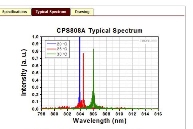
Spectrum of the CPS808A Diode Module taken at 20 °C, 25 °C, and 30 °C. The measurement was taken using Thorlabs <u>OSA201 Spectrum Analyzer</u>, which has a resolution of 7.5 GHz (0.25 cm<sup>-1</sup>).
