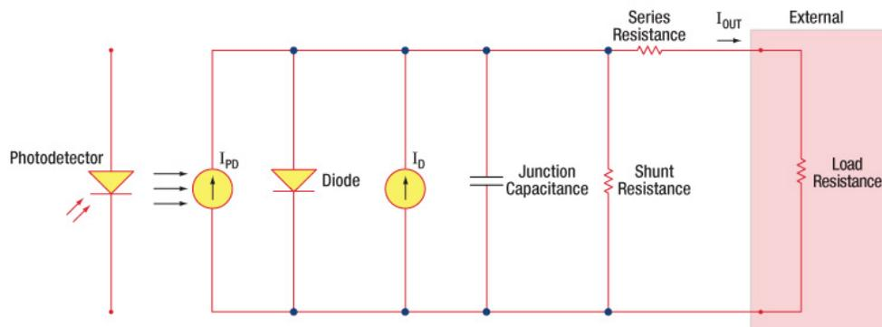
Figure 1: Photodiode Model
