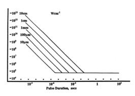
LIDT in linear power density vs. pulse length and spot size. For long
