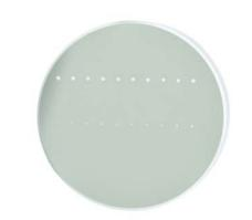
The photograph above is a protected aluminumcoated mirror after LIDT testing. In this particular test, it handled 0.43 J/cm<sup>2</sup> (1064 nm, 10 ns pulse, 10 Hz, Ø1.000 nm) before damage.
