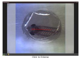
The Sample Monitor can be used to define the scan pattern using the "Draw and Scan" feature.
