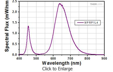
Broadband LED Spectrum Scaled to Min Power
