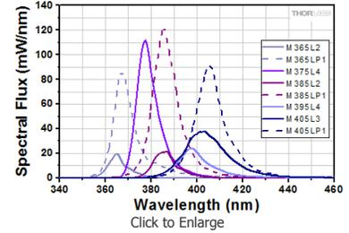
Visible LED Spectra Scaled to Min Power
