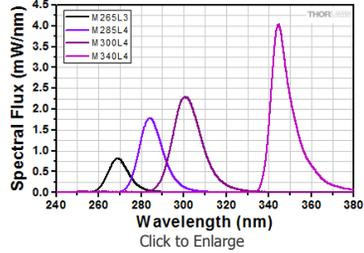
UV LED Spectra Scaled to Min Power
