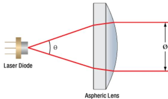
$\text{Ø}$  = Beam Diameter     $\Theta$  = Divergence Angle
