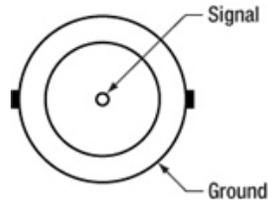
50  $\Omega$  Recommended Termination. For max output, please see detector drawings below.
