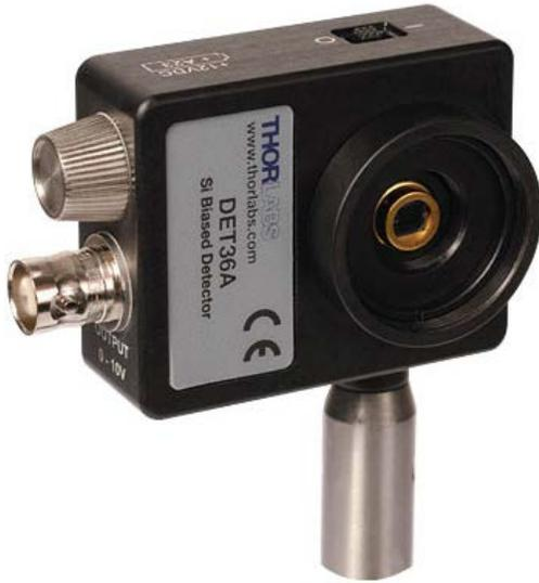
DET series detector mounted horizontally on a TR series post. Notice how the on/off switch is easily accessible from the top and the electrical connection comes in perpendicular to the beam path.
