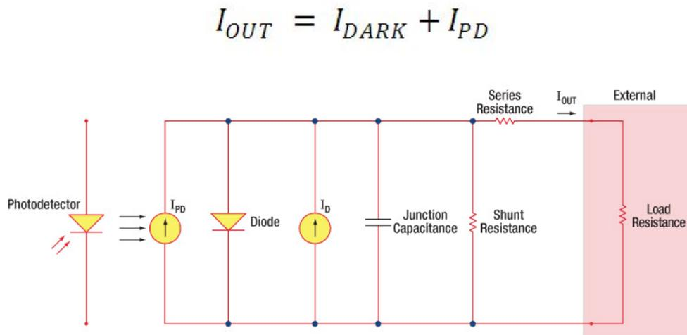
Figure 1: Photodiode Model
