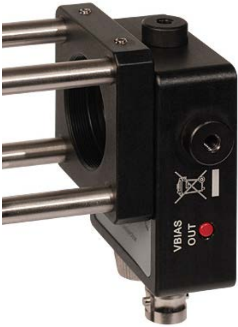
This picture shows a DET series detector attached to a CP02 cage plate after removing the SM1T1. The retaining ring from the SM1T1 was used to make the orientation of the detector square with the cage plate.
