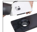
Click to Enlarge This photo shows the male D1N dovetail on the trinoculars next to the female D1N dovetail on the epi-illumination arm.
