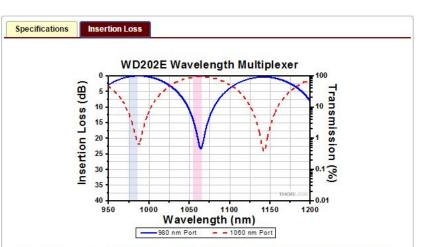
This plot shows an example of the spectral performance of a 980 nm / 1060 nm WDM. The lines represent the spectral response of each channel, while the blue and red shaded regions denote the bandwidth around each channel. This data is typical; performance of each coupler may vary within the coupler specifications. Data was obtained without connectors.
