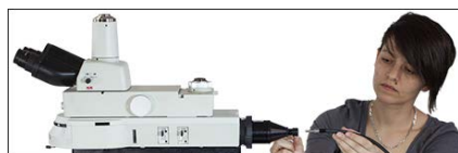
Click to Enlarge Here, a liquid light guide lamp is being connected to the epi-illuminator module via a bayonet-to-LLG adapter.
