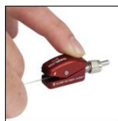
Click to Enlarge Step 2: Feed Fiber Through the Connector
