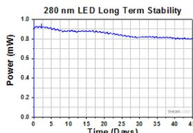
The M280L3 LED has a typical lifetime of  $>500$  hours. In this case, the unit under test had dropped to  $\sim 80\%$  of the initial output power after 45 days.
