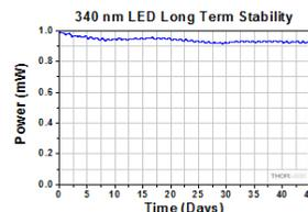
The M340L3 LED has a typical lifetime of  $>3,000$  hours. In this case, the unit under test continued to provide more than 90% of its initial power after 45 days.
