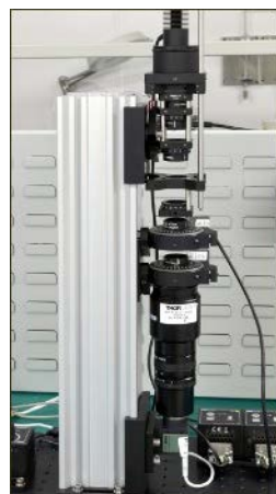
Click to Enlarge Custom Liquid Crystal Cell Test Setup
