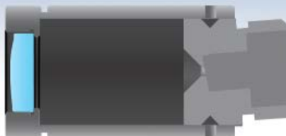
Fixed Focus Collimators Contain One Factory-Aligned Aspheric Lens
