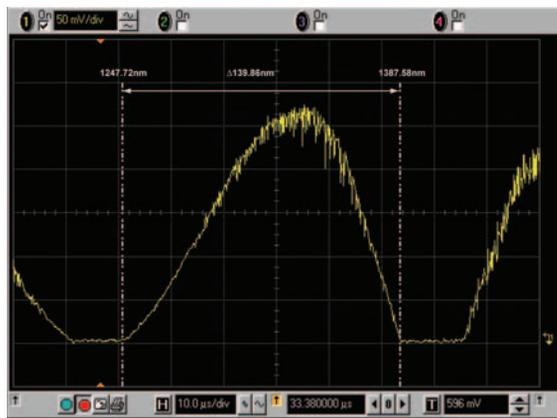
Figure 2: The Power Monitor signal accessible from the rear panel shows optical power as a function of time.
