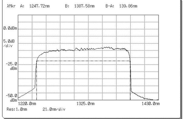
Figure 3: Spectrum of the (SL1325-P16) swept laser showing an active wavelength tuning range of 155nm centered around 1325nm.
