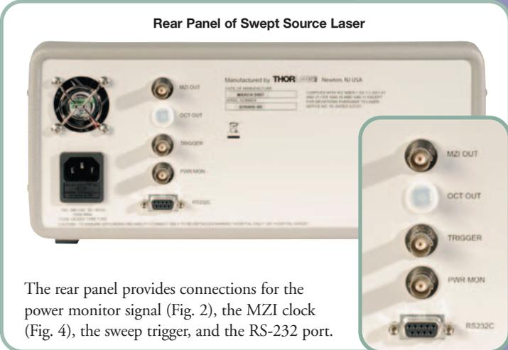
The rear panel provides connections for the power monitor signal (Fig. 2), the MZI clock (Fig. 4), the sweep trigger, and the RS-232 port.
