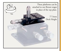
The ATP001 and ATP003 tilt platforms provide  $\pm 4^{\circ}$  of both pitch and yaw adjustment. They are designed specifically to offer a low-cost, five-axis solution when used in conjunction with the NanoMax<sup>TM</sup>, RollerBlock<sup>TM</sup>, PiezoBlock<sup>TM</sup>, or MicroBlock<sup>TM</sup> stages. The optical axis height is then raised by 15mm to 90mm when mounted directly on the stage.
