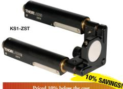
The KS1-ZST combines our traditional KS1 kinematic mount with our ZST13 stepper motor actuator. By using the same body as our standard KS1 kinematic mount, the KS1-ZST works as a drop-in replacement when automating an optical setup. Additionally, the motorized actuators enable finer, more precise positioning than possible with manual adjusters. Integrated electromechanical limit switches prevent damage if the actuator is over driven, while providing homing better than 15arcsec.
