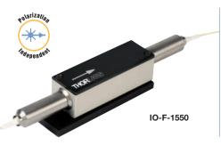
The IO-F-1550 and IO-F-1550APC are polarization-independent fiber isolators designed for use in the 1530 to 1570 nm range with powers up to 5 W. Returning light is displaced from the optical axis, resulting in 32 to 38 dB of isolation. Due to the polarizationindependent nature of these isolators, the insertion loss and the isolation value will not change with respect to the input or returning light's state of polarization.
