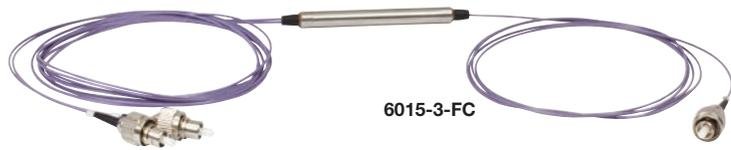
This fiber optic circulator is a non-reciprocating device that transports an optical signal from one port to the next port but only in one direction (i.e., 1 → 2 or 2 → 3). They may be used to separate forward and backward propagating signals, typically with 45 dB of isolation and a directivity (crosstalk) figure of better than 50 dB. These circulators are available unconnectorized or with either FC/PC or FC/APC connectors on both ends.
